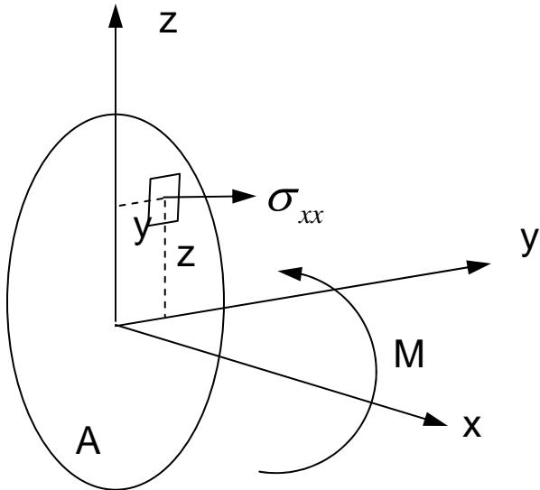
$$\int_A \sigma_{xx} dA = 0 \quad \Rightarrow \quad \int_A z dA = 0 \quad \text{neutral axis is at centroid}$$
